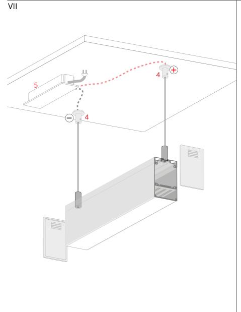
Suspend the lighting fixture from the ceiling fasteners (4) which are connected to the power supply (12 V / 24 V) (5).
